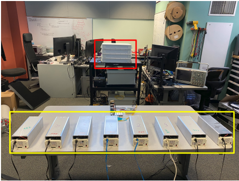
Figure 5: Our RRU hardware setup including a 64-antenna Faros base station, shown in a red box, and eight Iris users, shown in yellow box, both from Skylark Wireless.
